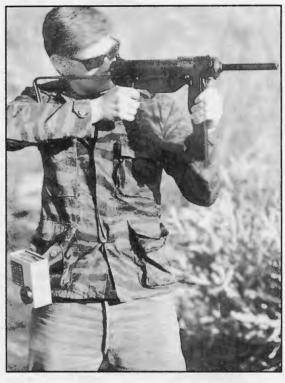
M3 "Grease Gun" chugs away at only 405 rpm. Shooter determines the cyclic rate of his full auto weapon and ammo combination with PACT™ MKIII attached to his side with belt clip.
